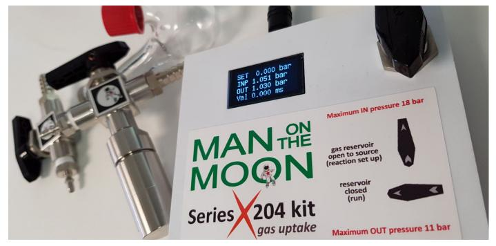
This device allows to feed reactions with gas, at the desired constant pressure in the range 1-10 bar(a), and monitors gas consumption along the reaction via the decrease of pressure in an internal reservoir. For pressure programing and data recording, the device must be connected via Bluetooth to a PC.
