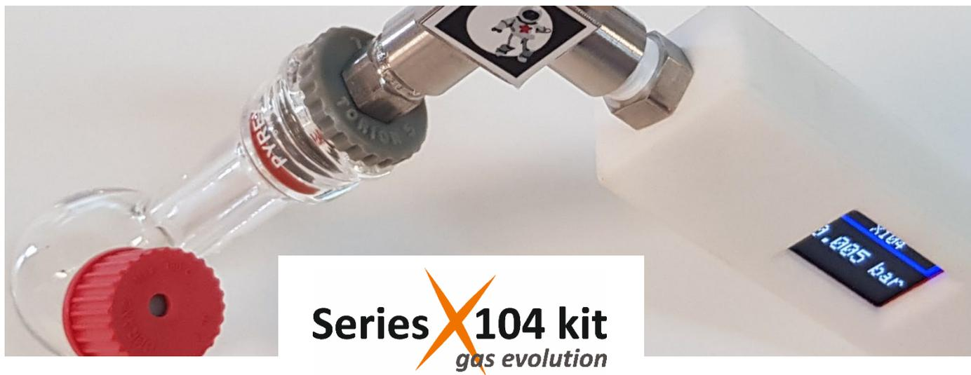
The device serves to monitor pressure variations within a closed reaction flask.
